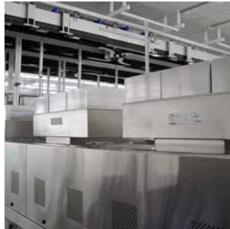
AMC filtration on top of process equipments
