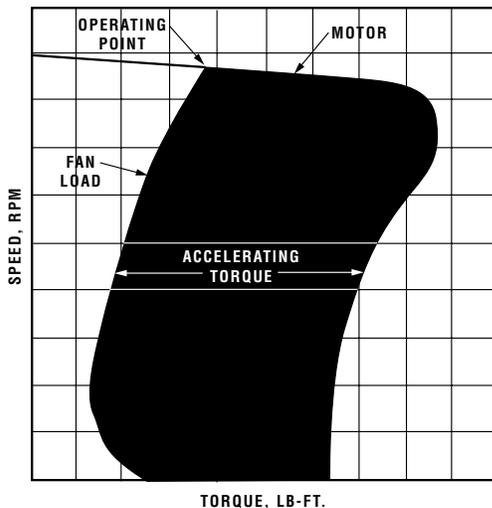
The shaded area represents the accelerating torque available at any speed. Fan speed torque curves are available from the fan manufacturer.
