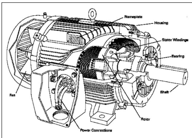
There is a broad range of types and sizes of motors manufactured and naturally not all are manufactured the same way, but they all incorporate the following similar basic components.
