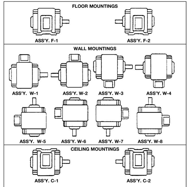
F-1 is most commonly used on the majority of fan applications, regardless of fan arrangement, mostly because of availability. Unless otherwise specified, NEMA assembly F-1 will be provided.
