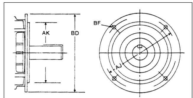
The Type C-face provides a male rabbet and tapped holes for mounting bolts while the Type D-flange provides a male rabbet and flange holes for through-bolts.
