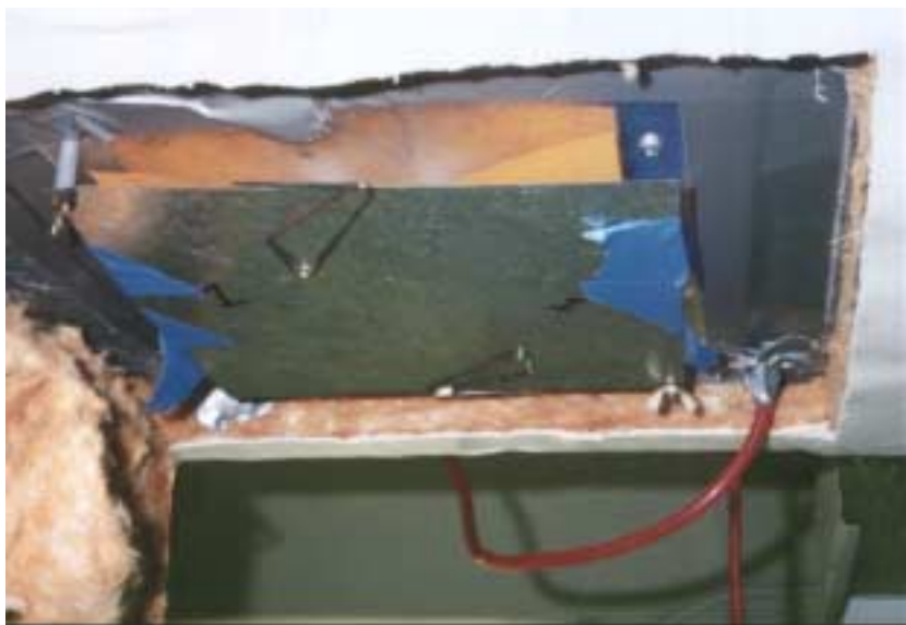
Figure 6. Impaction plate installed in Building LS-2
