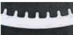
Configuration of the finned heat-transfer tube
