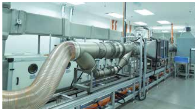
Filter test rig in Camfil Malaysia
