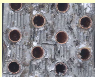
Unprotected coil after 4000 hours, diagonal section
