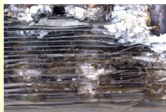
Unprotected coil after 4000 hours, fin edges
