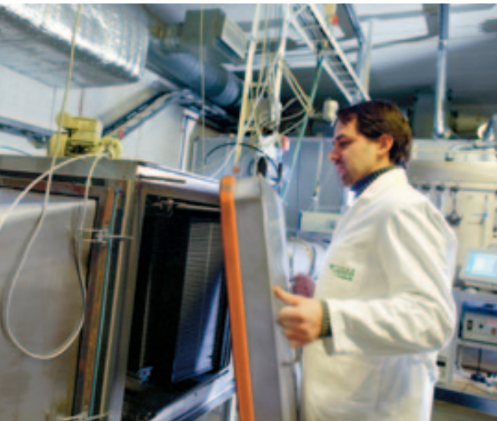
Molecular filter test rig.
