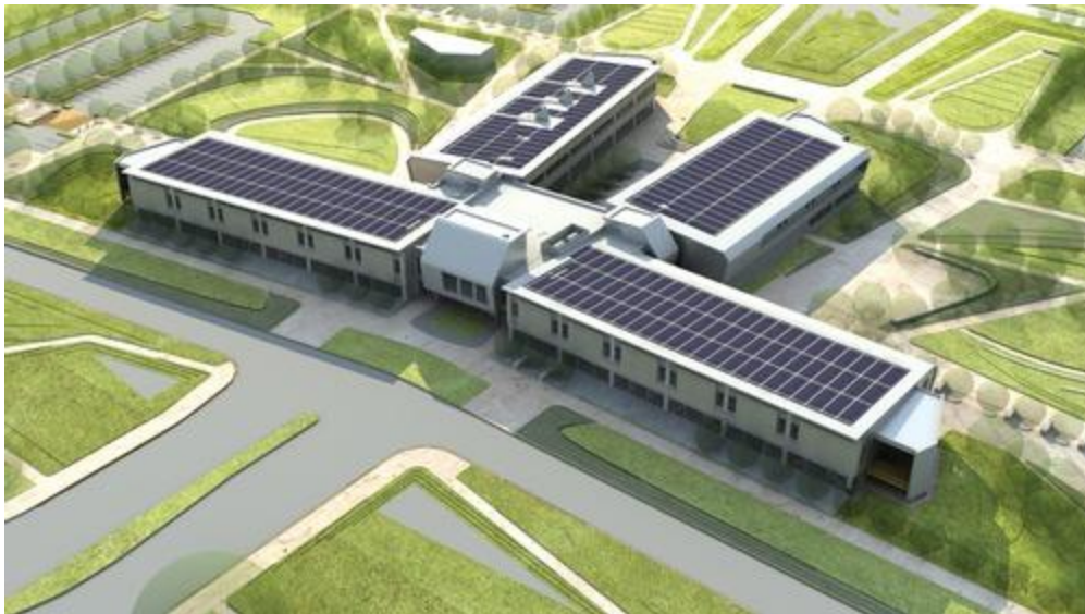
Figure 20. Example of PV Installation at Ohlone College, Newark Center, Newark, CA: 450 kW, 38,000 ft 2 (Esberg 2010)
