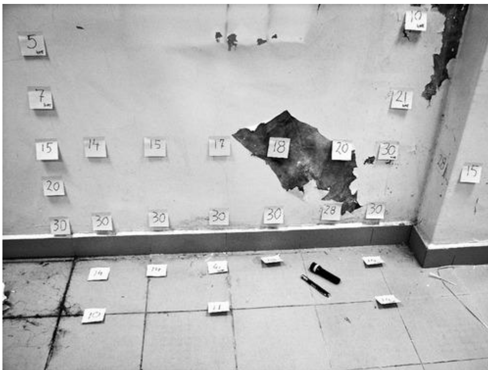
Figure 12. Example of Documenting Both Values and Pattern of Moisture
