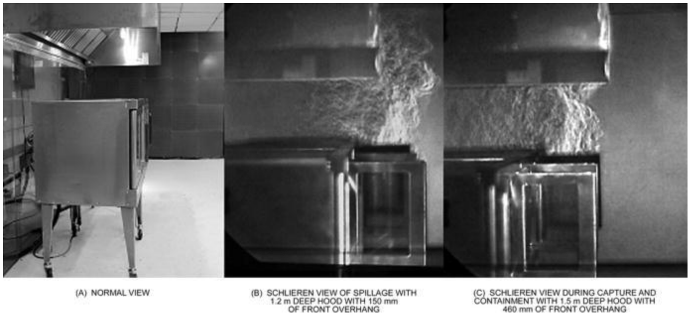
Figure 10. Three Ovens under Wall-Mounted Canopy Hood at Exhaust Rate of 1600 L/s (Swierczyna et al. 2006)
