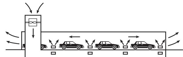
FIGURE I.3.1(b) Semitransverse Supply Ventilation System.
