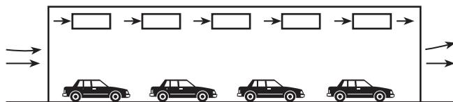
FIGURE I.2.1(c) Longitudinal Ventilation System with Jet Fans.
