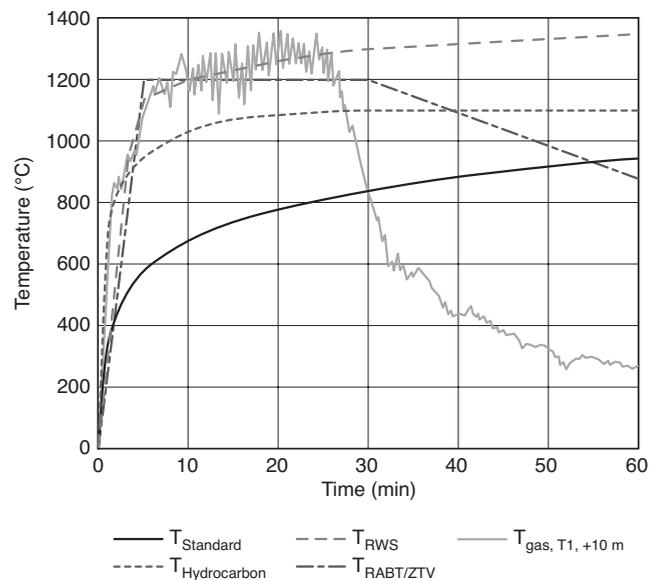
FIGURE A.7.3.2(b) Test Fire Curves.
