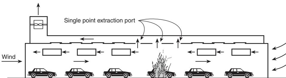
**FIGURE I.4.2 Single Point Extraction with Jet Fan Longitudinal Ventilation Support.**
