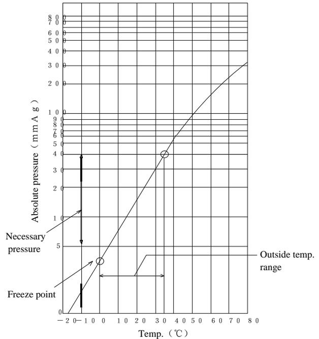
(Example) In the case of ambient temperature 7.2 °C, vacuum drying is impossible unless the pressure is reduced to -8mmHg or less. So, “selection and maintenance of a vacuum pump” is important for vacuum drying.
