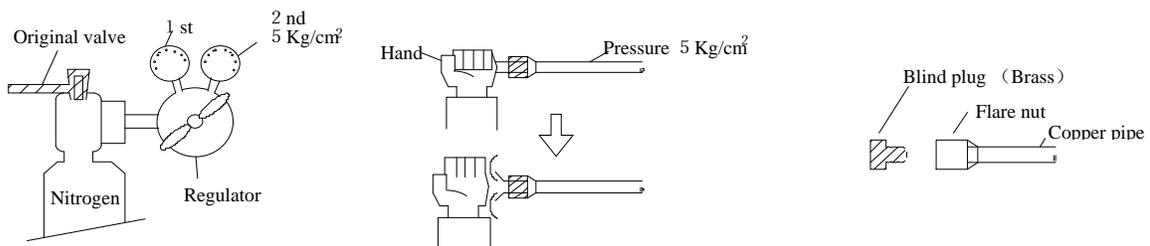
(When flushing, put a waste cloth at the end of the pipe in order to check the foreign substances and the amount. If moisture is detected even in a small amount, remove the moisture in the pipe completely)
