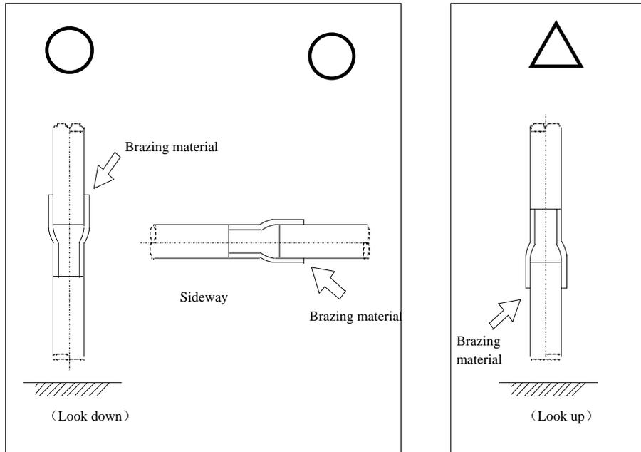
b) Be sure to use specified liquid pipes and gas pipes. Take care of fitting direction and angle. (to prevent oil return and drift)---case examples (see p.53)
