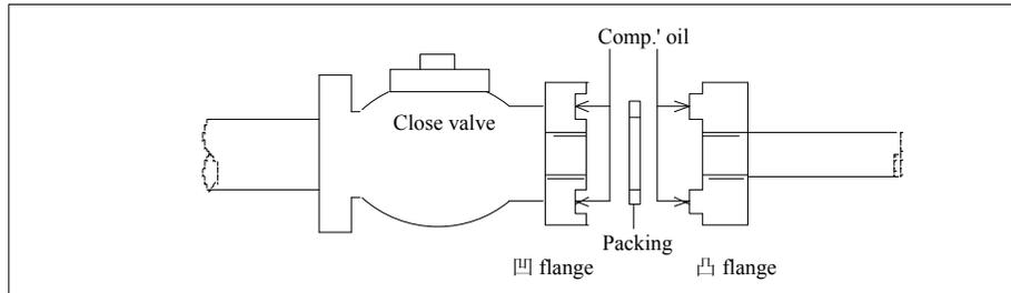
c) Tighten bolts in a diagonal line in sequence in order to evade impartial tightening.
