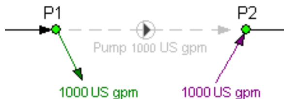
Figure 119 Fixed Flow Rate Pump replacement
