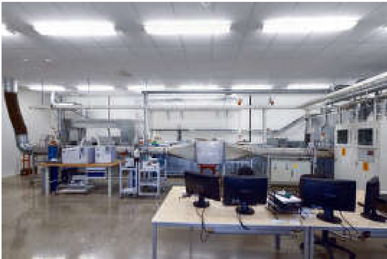
Molecular filter test equipment according to ISO 10121
