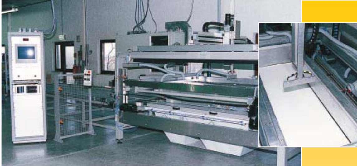
Camfil Farr laser Scanner test for production control and classification of Absolute filters.
