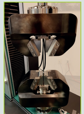
Hydraulic wedge grips, software controlled in support of automation
