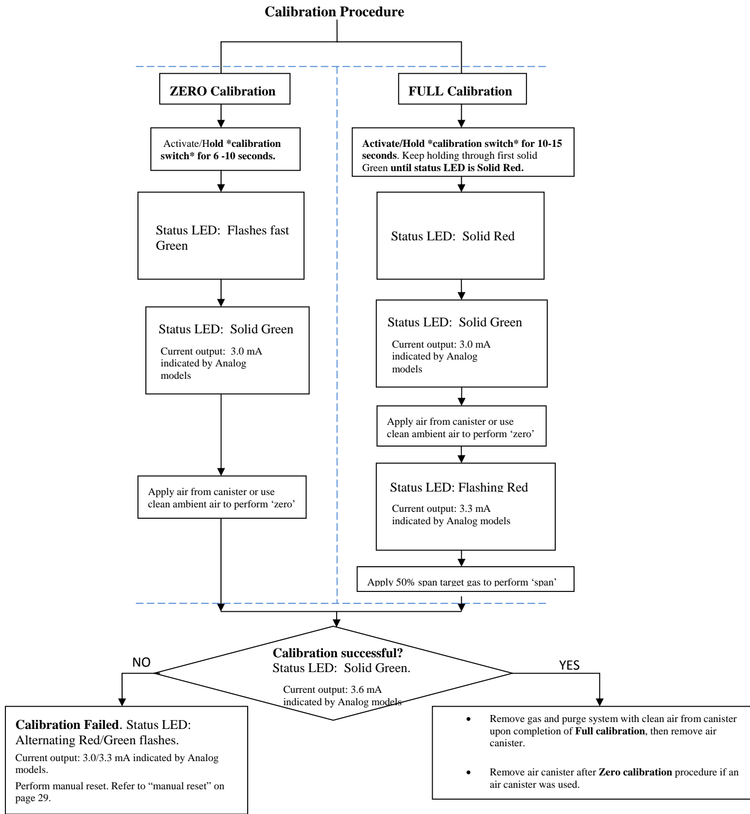
Figure 16: Calibration flow chart
