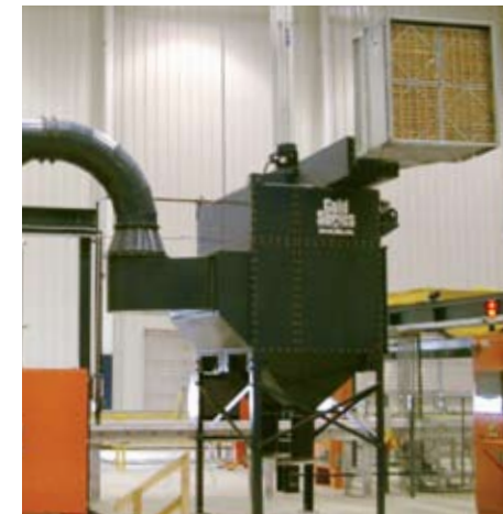
Abrasive Resistant Inlet, Top Mount Fan, Silencer, & Safety Monitoring Filter
