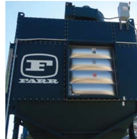
Explosion Vent-ATEX Approved Rupture Panel
