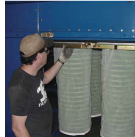
Overbag Option for Fibrous Dusts like Paper & Fiberglass
