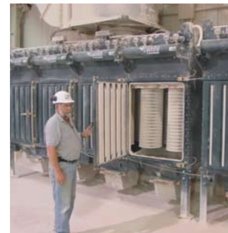
Louvered door inlet for cross-flow applications
