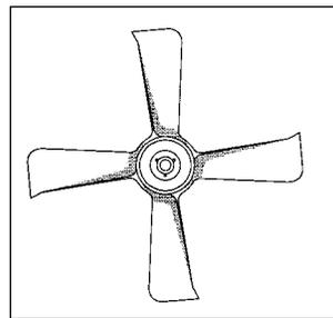
Figure 6. Medium Width Stamped Steel Impeller
