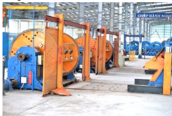
Rigid Type Stranding M/C 630Φ/(12B+18B), Side loading type Range: ID 22Φ/ OD 55Φ
