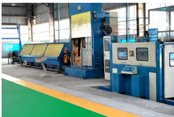
Rod Breakdown Drawing M/C Range: 1.35mm - 3.5mm
