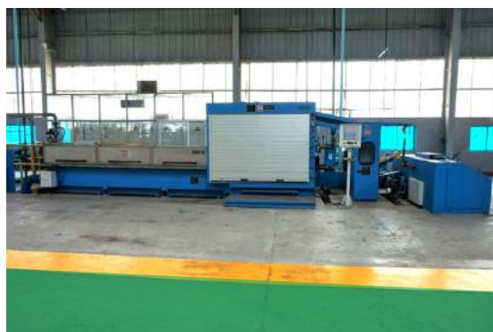
Intermediate Multi Wire Drawing M/C Range: 0.28mm - 1.05mm
