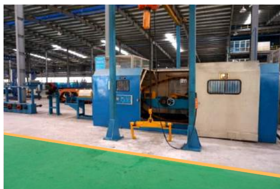
Double Twisted Bunching M/C (1250Φx80Φx950Φ) Range: Out diameter less than 20mm
