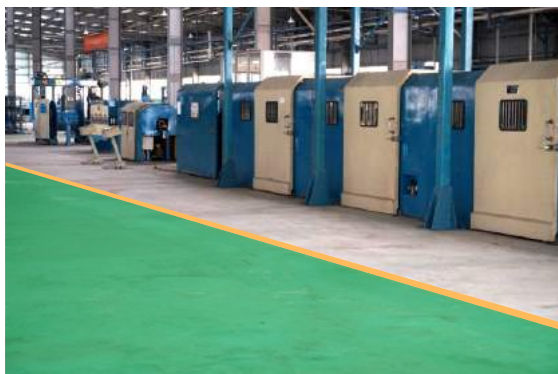
Skip Type Cabling M/C (1250Φ x 80Φ)x(3Bow +1) Range: Max~19ΦOD(150sq)x4C
