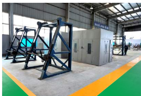
Wire Braiding M/C 16, 24 & 32 Carrier
