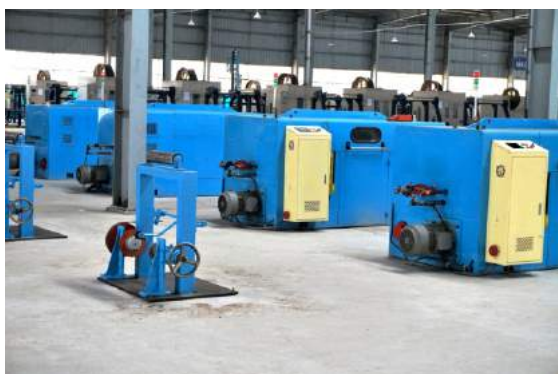
Double Twisted Bunching M/C (650Φ x 127Φ) Range: 0.3mm - 6.0 mm
