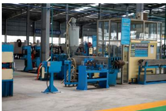
Plastic Insulation & Sheath Extrusion Line (Screw 90Φ & 120 Φ)
