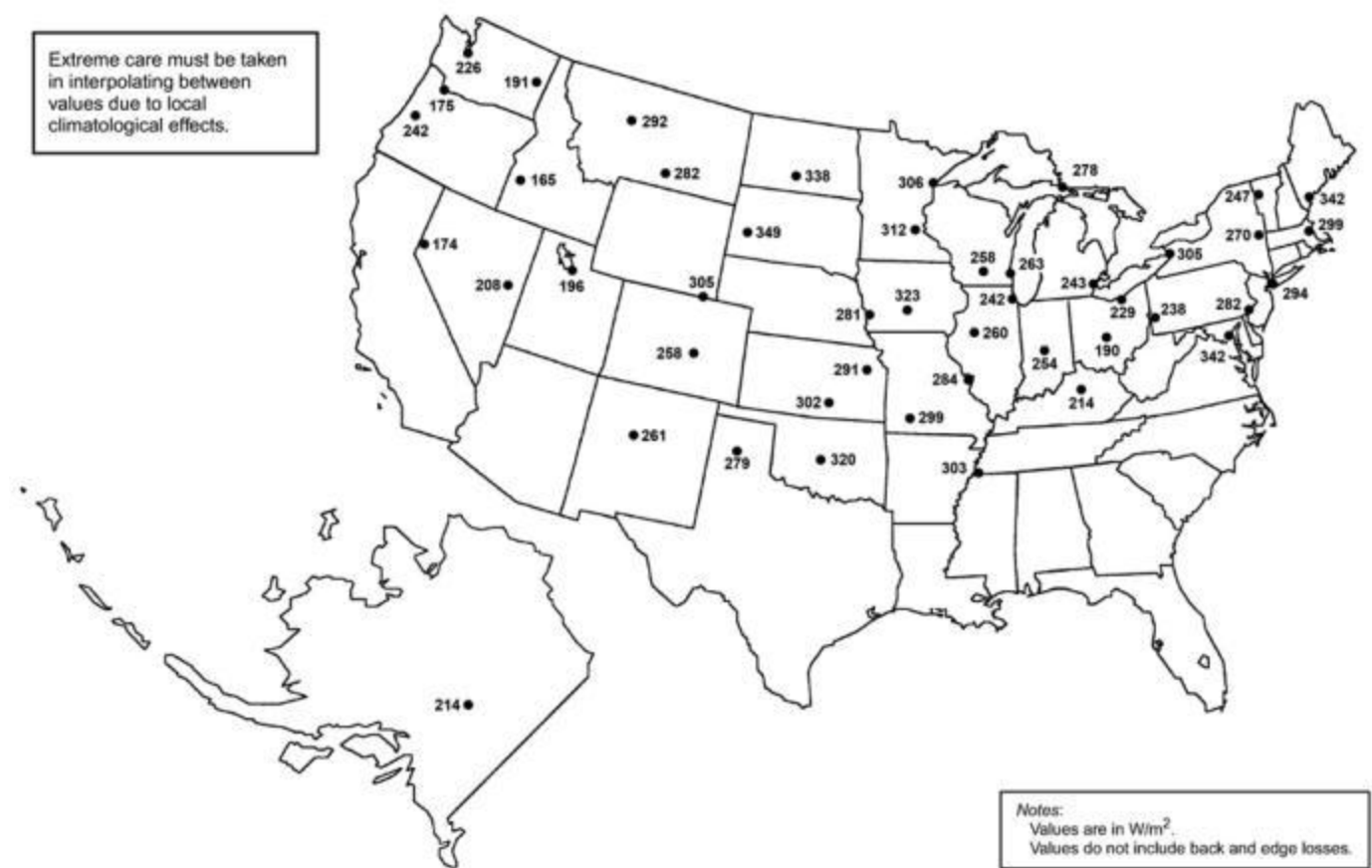
Figure 1. Snow-Melting Surface Heat Fluxes Required to Provide Snow-Free Area Ratio of 0.5 for 90% of Snowfall Hours at That Location
