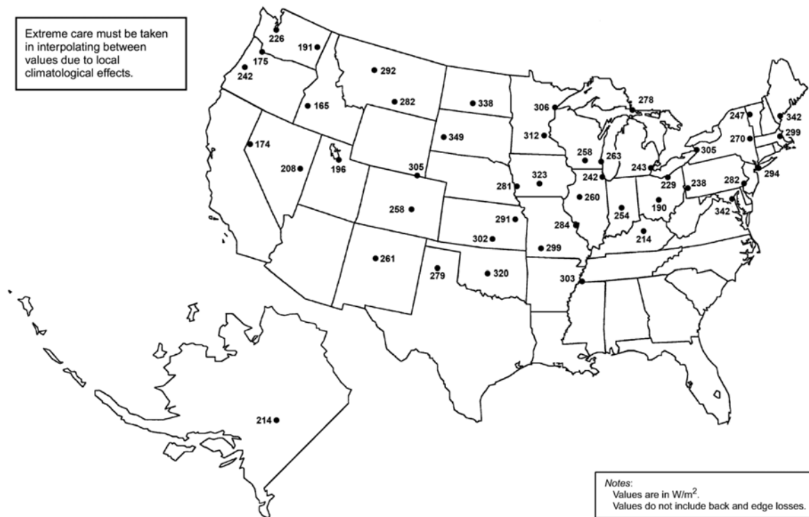
Fig. 1 Snow-Melting Surface Heat Fluxes Required to Provide Snow-Free Area Ratio of 0.5 for 90% of Snowfall Hours at That Location
